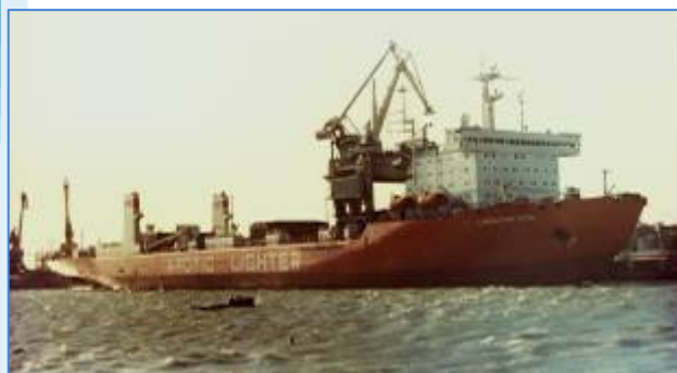
Nuclear powered transporting vessel of ice-breaking type “SEVMORPUT” Deadweight: 33 780 tons Totally built: 1 vessel
